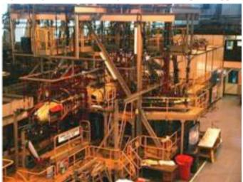
specimen looking for cracks. If something is found it is first logged and then assessed. If the crack is big enough the fleet of aircraft would be grounded but this is incredibly rare. Much more likely an instruction would be sent out to look at that location in the fleet of flying aircraft and report back. In the more serious cases the offending component would be changed. My friends at BAe Systems have kindly sent me
