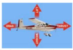
So what happens if the pilot closes the throttle a bit? Thrust gets smaller and the aircraft slows down until drag equals thrust again. But since the aircraft is slower, lift is lower but weight stays the same. So the aircraft goes down! What the pilot can do is raise the nose to get more lift. This will only work until the nose is raised to 15° or so. The aircraft then stalls and the aircraft must go down unless the pilot opens the throttle again!
