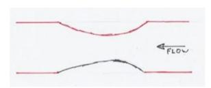
Now I have produced a drawing for you. This shows a square pipe with a constriction in it and is viewed from the side. It is what is called a venturi. Bernoulli realised that the energy of the air all the way down the pipe has to stay the same. For the air to get past the constriction it has to flow faster and to
